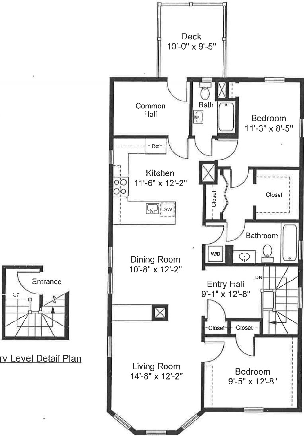
Unit 3 Floor Plan Ceiling Height = 9'-1"
